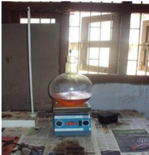
Fig.5 Separation of Methanol from Esterified Oil
