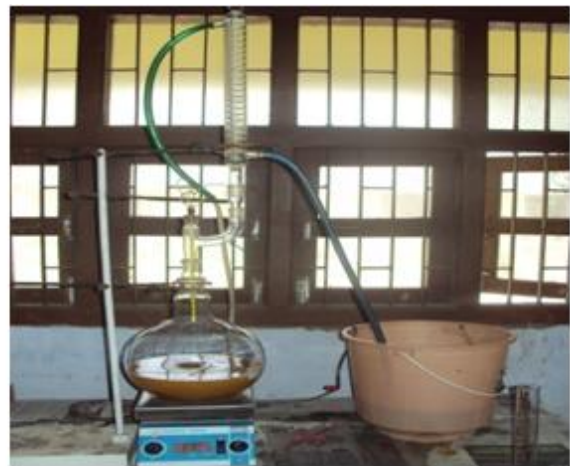
Fig. 2 Esterification Process Using Acid Catalysis
