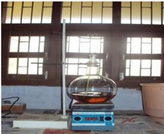
Fig. 1 Pre-heating of Raw oil
